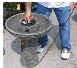
Pull out cord slack, set pump in housing
