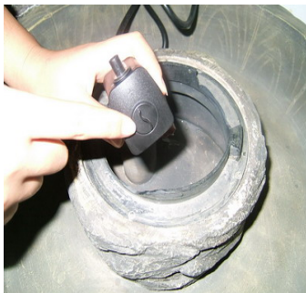
Set pump flow to 3/4 strength
