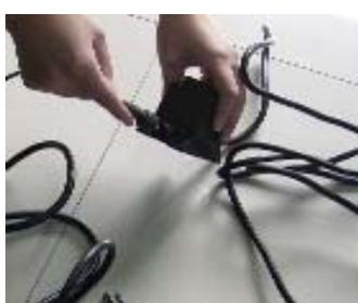
Attach the light cord to the transformer.
