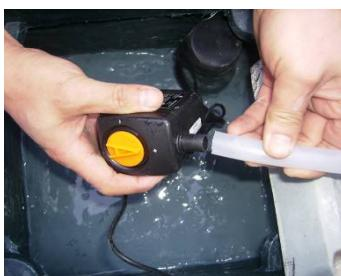
Connect the tubing to the pump and adjust the pump to your desired setting.
