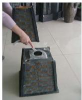
Feed the tubing from the top section through the opening of the middle section as shown.
