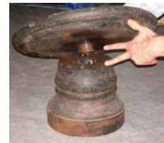
Place the pump housing/riser on a flat surface. Set the middle plate on to it by aligning the groove as shown.
