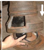
The next step may require 2 people. Lift the assembled top, middle plate and pump housing/riser. Carefully rest or hold the assembled parts while you feed the light cord down the cord pipe. Gently set the assembled pieces down over the collar and into place by aligning the groove as shown (above right). We suggest aligning the grooves prior to lifting the assembled pieces so that is easier to line them up when lowering into place.
