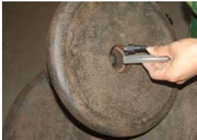
Pass the tubing and light cord through the opening in the top plate as shown.
