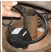
The next step may require 2 people. Lift the assembled top, middle plate and pump housing/riser. Carefully rest or hold the assembled parts while you feed the light cord down the cord pipe. Gently set the assembled pieces down over the collar and into place by aligning the groove as shown (above right). We suggest aligning the grooves prior to lifting the assembled pieces so that is easier to line them up when lowering into place.
