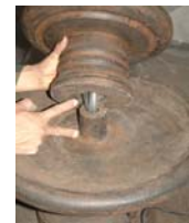
Set the top in place by aligning the groove as shown.
