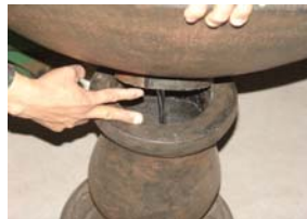
Carefully place the bowl on to the pedestal by aligning the grooves as shown above.
