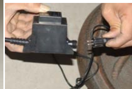
Attach the light cord to the transformer as shown.
