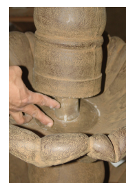
The riser is installed next. After feeding the tubing through the riser, slide it in place with the grooves aligned.
