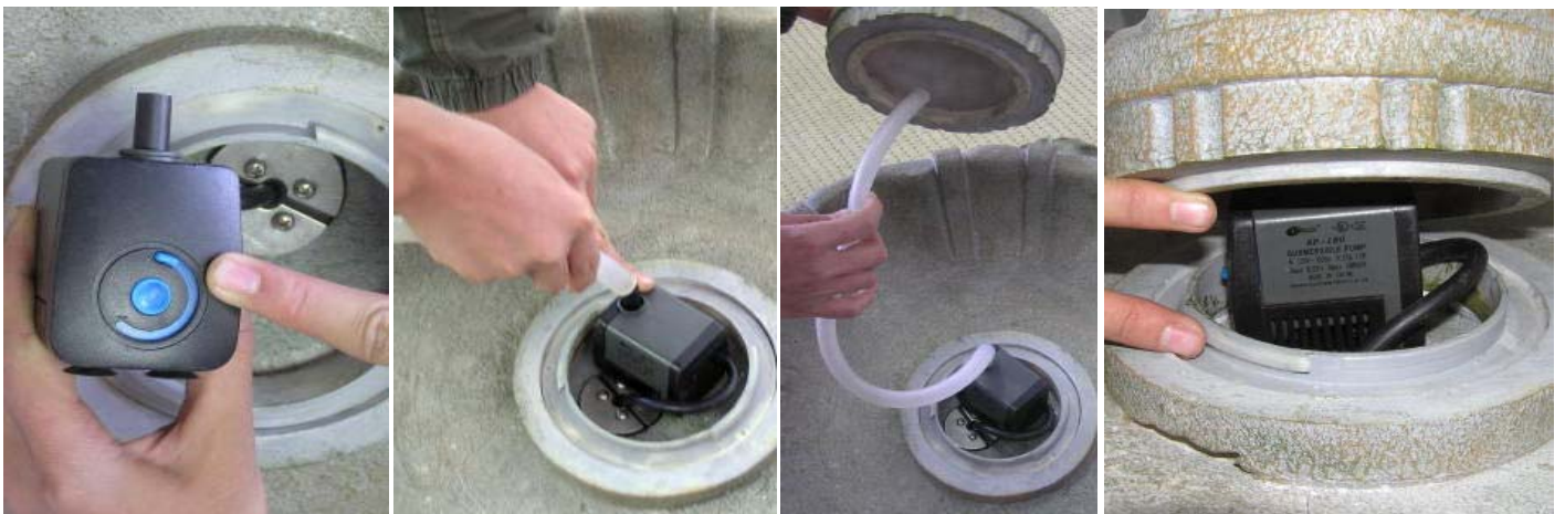
Pump is preinstalled with cord seal. We suggest setting flow to full strength for best effect. Pump should sit flat on bottom. Attach hose, feed through riser, and secure into place.
