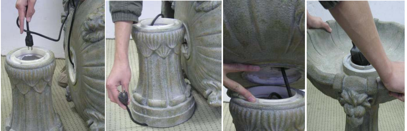
Run pump cord through standpipe and base, place in groove at bottom. Secure bowl to base.
