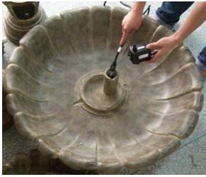
Feed the pump cord through the cord pipe.
