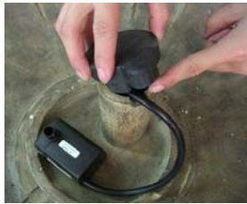
Place the cord pipe cover over the cord pipe as shown above.
