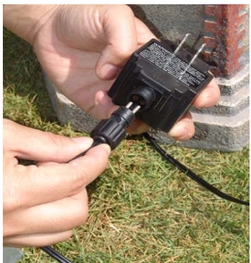
Attach the power cord to the transformer.
