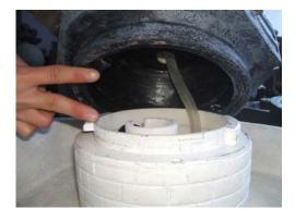
Attach the tubing to the pump securely. Verify that the tubing is the proper length to allow the pump to sit firmly at bottom of the reservoir without bending, because this could reduce the water flow. It may be necessary to trim the tubing to the proper length.
