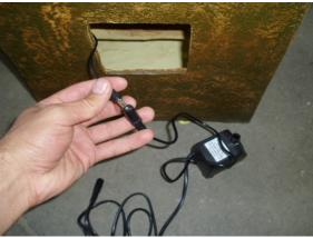
Connect the pre installed light cord to the transformer.
