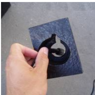
Run the light cord through the hole in the pump access door and out the back access hole.
