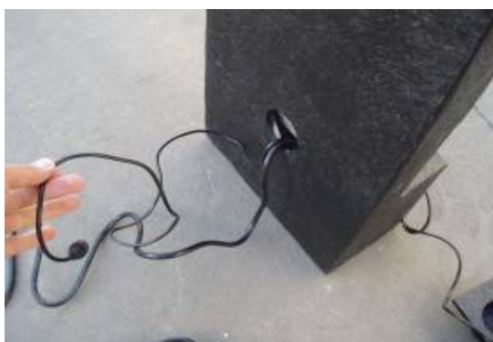
Run the light cord through the hole in the pump access door and out the back access hole.
