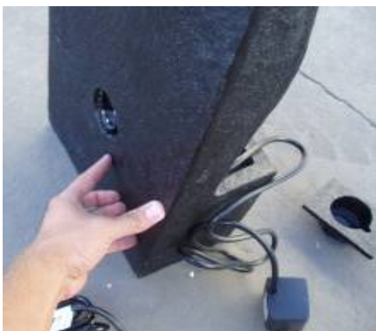
Run pump cord out access hole on the back.
