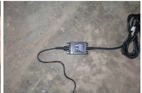
Attach light cord to transformer. Be sure it is tight. Place transformer in a secure area, preferably under cover. While this unit is rated for outdoor use, it should not be fully submersed in the water.
