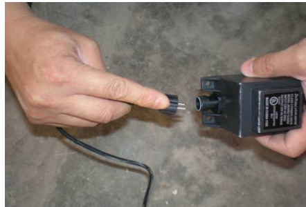
Attach light cord to transformer. Be sure it is tight. Place transformer in a secure area, preferably under cover. While this unit is rated for outdoor use, it should not be fully submersed in the water.
