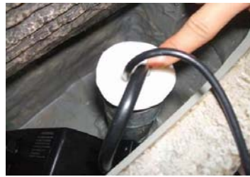
Insert rubber bung as shown.
