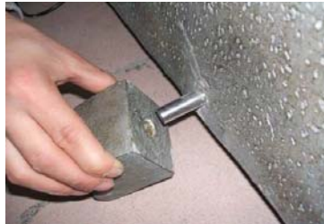
To use optional stabilizing system: Insert pins and turn clockwise until tight. Slip leg over pin until firm against back of fountain. Repeat for the other leg.
