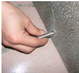
To use optional stabilizing system: Insert pins and turn clockwise until tight. Slip leg over pin until firm against back of fountain. Repeat for the other leg.
