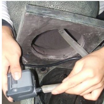
Connect tubing to the pump
