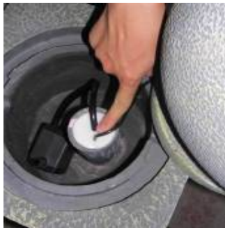
Insert rubber stopper as shown.
