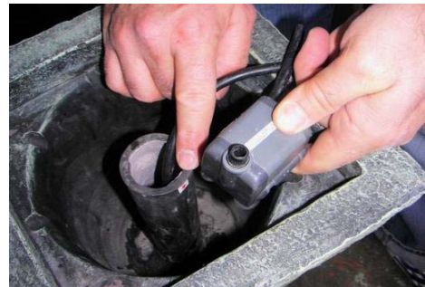
Be sure pump line up with arrow for proper fit at bottom of reservoir
