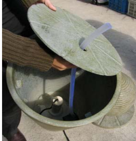
Sit pump at bottom, slide tube through baffle plate as shown.
