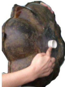
Insert the "slip fit" pipe into the middle bowl as shown.
