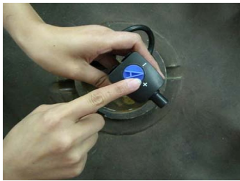
For ideal operation, the pump is preset to 1/2 strength. Adjust as needed.
