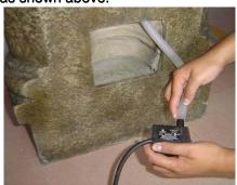
Attach the tubing from the feature to the pump. Adjust the pump to your desired setting and place inside the reservoir so that it will be fully submersed.
