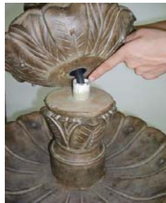
Slide the final bowl and top into place
