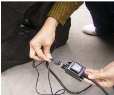
Attach the cord to the transformer. Ensure it is tight.
