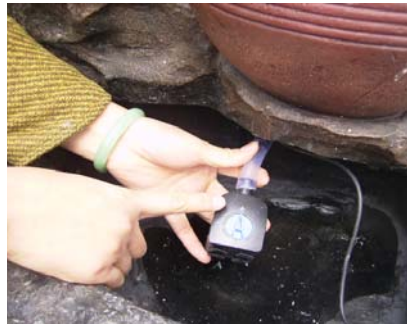
Pump is set to full. Reduce flow if lower splash is desired.
