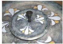
The spray nozzle head should look like this. Adjust the flow and the height of the nozzle by tightening or loosening the head slightly.
