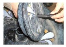
Go the tube into the hole of pump cover and then inset the nozzle head into it
