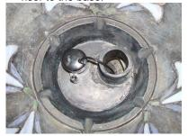
For the solar powered pump, sit the pump centered in the cavity.
