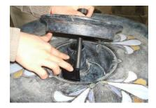
Connect the nozzle to the pump
