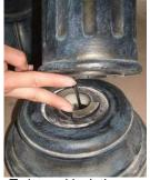
Twist and lock the riser to the base.
