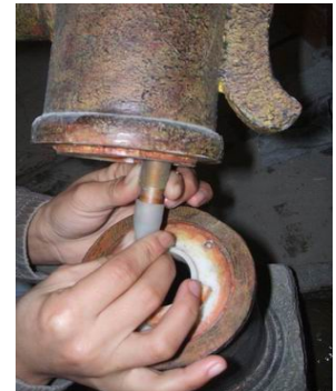
Connect the tubing to the top section by metal slip fit.
