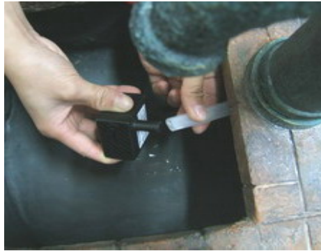
Connect the tubing to the pump.
