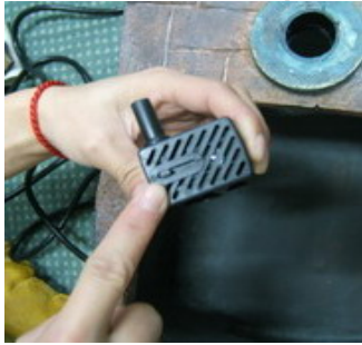
Pump is set to full. Reduce flow if lower splash is desired.
