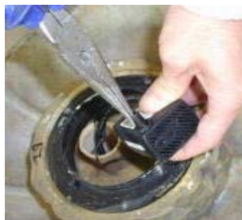
pull pump outlet out with pliers
