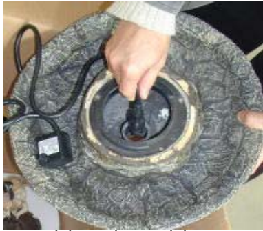
cord through standpipe
