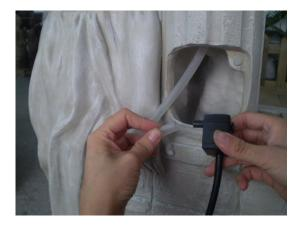
Connect the tubing to the pump. The pump should sit flat inside the housing without any kinks in the tubing.
