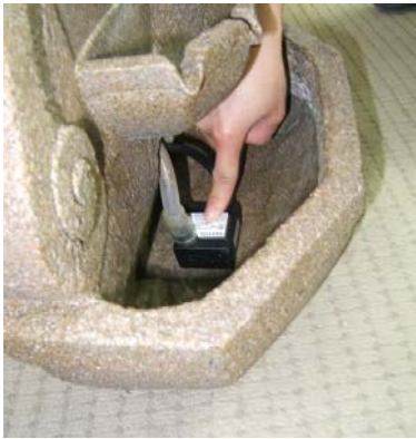
Place pump in housing be sure not to kink hose
