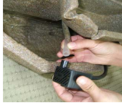
Connect the tubing to the pump
