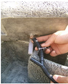
Connect the pre-installed tubing from the "Y" connection to the metal fitting. Connect the tubing from the top to the remaining output of the "Y".
