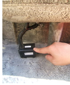
Place the pump inside the housing, ensuring the tubing is not kinked.
