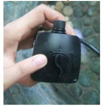
Adjust the pump to the desired setting. We recommend the max setting but this can be adjusted depending on the application.
