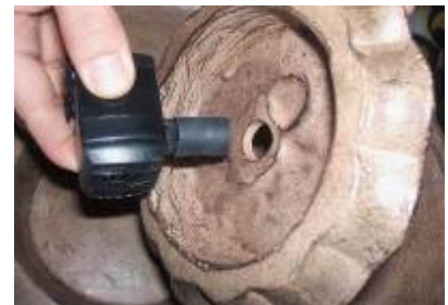
Put the nozzle into the pump cover. (short nozzle shown)
