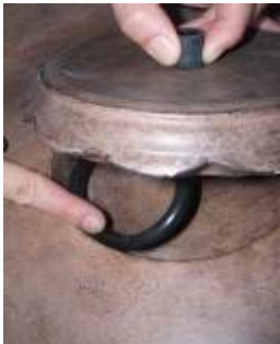
Set the pump cover into place and make sure the nozzle is straight.
