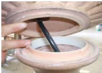
Twist and lock the bowl to the riser.
