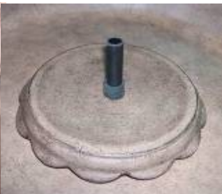
Set the pump cover into place and make sure the nozzle is straight.
