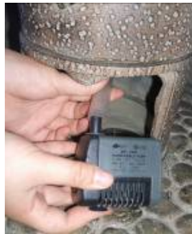
Connect the pump to the tubing.
