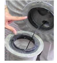
The power cord is inserted through the pipe in the bowl as shown.
