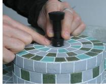
Insert nozzle through rubber stopper, then into hole of pump cover. Place cover over housing noting the grooves for proper fit.
