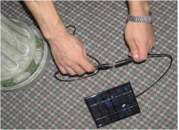
For solar pump, attach cord to panel, and stake firmly into ground.
