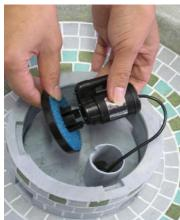
For solar pump, attach filter on bottom. Chosen pump must be centered in cavity.
